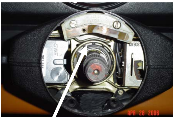
Steering wheel column bearing with retainer - Check for wear here by moving shaft.
